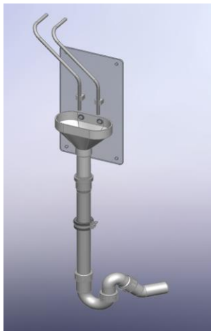
Figure 5. Schematic figure of a free drainage.
